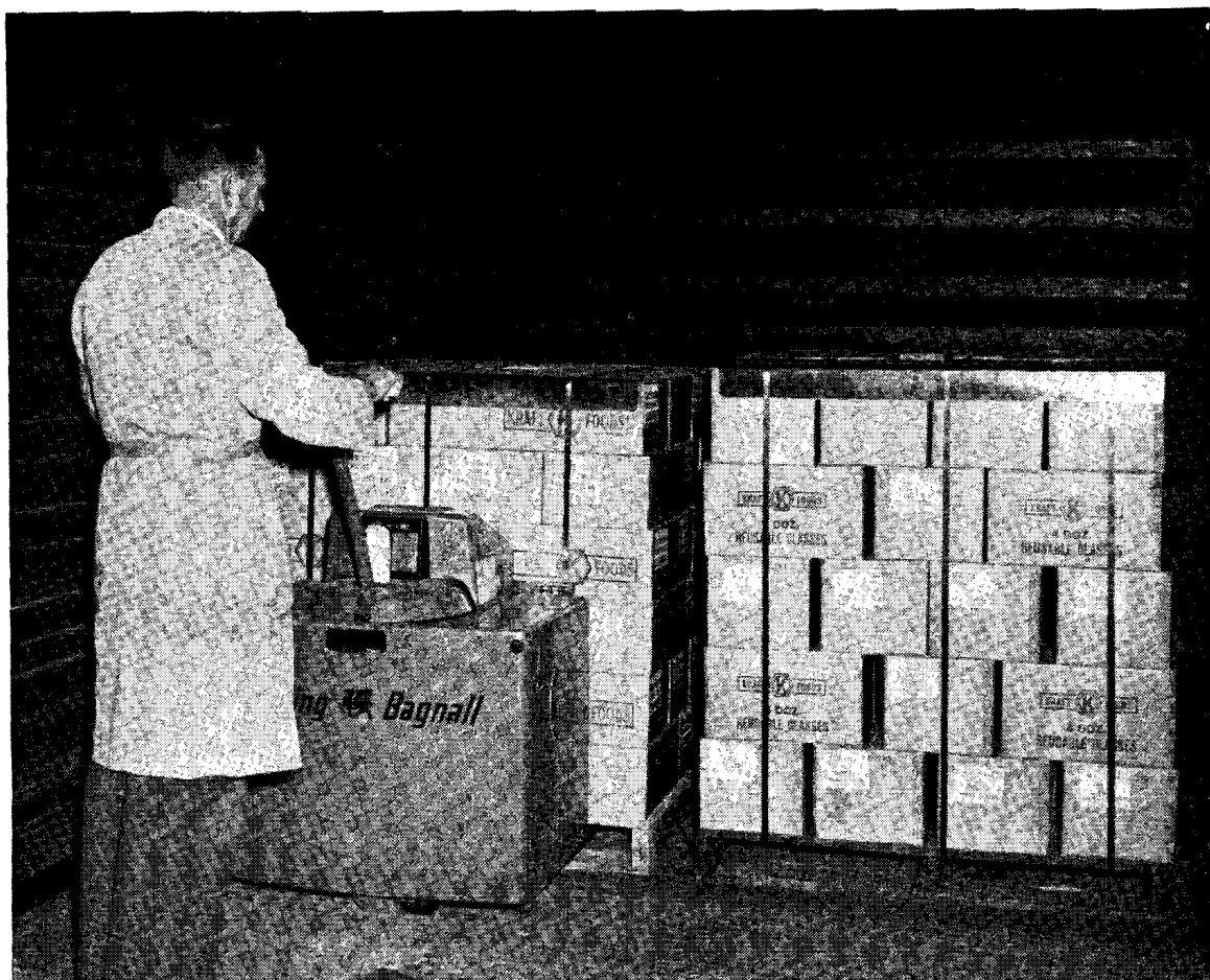
Loading with a pedestrian palletiser.
